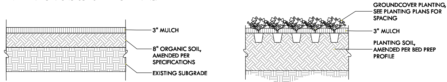
TYP. PLANTING SOIL PROFILE DETAIL N.T.S.
