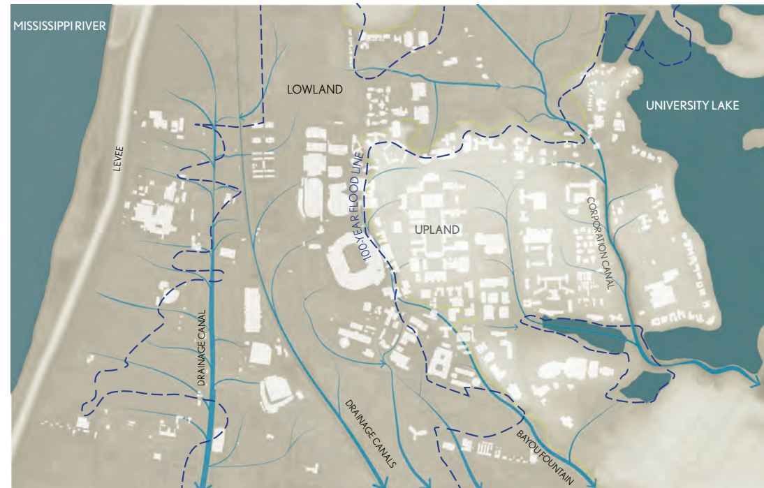
Mapping of drainage ditches and water bodies from GIS and satellite imagery.
