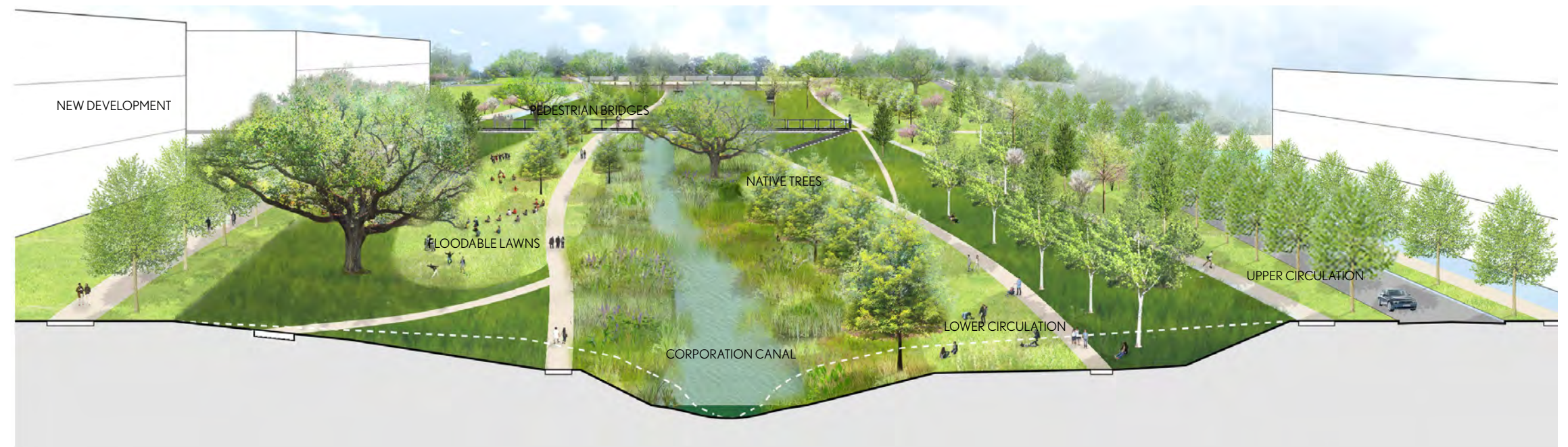
The Master Plan vision for Corporation Canal features all three strategies included in the storm water management framework. Native wetland vegetation planting along widened canal banks helps to slow water by creating more opportunities for infiltration and transpiration before entering the canal; broad lawns mid-bank create spaces for storm water to be stored during major events; all while the critical flows and ability to drain water from across the watershed are maintained.
