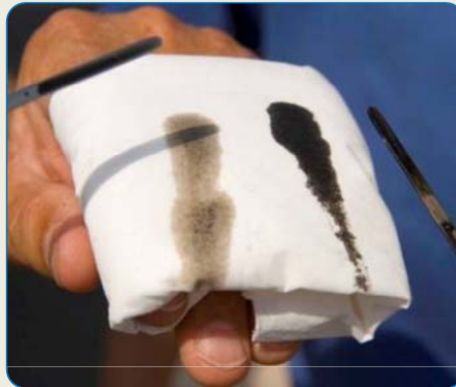
The oil from the Toyota fuelled by GTL diesel compared to the oil from the Toyota running on normal diesel after the GTL challenge
